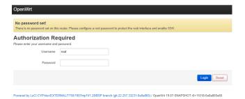
Note: once login is successful, it is recommended to set the password first for securing the web interface. Go to System -->
